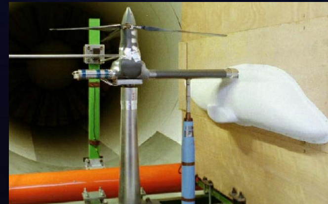
ONERA wind tunnel model (Desopper 2002)
