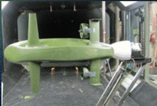
Subscale wind tunnel model of an early variant of the CCH airframe at - 90° angle of attack
