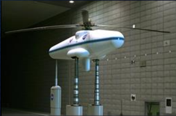
UH-60 rotor on the LTA in the NASA/Ames 80x120 wind tunnel
