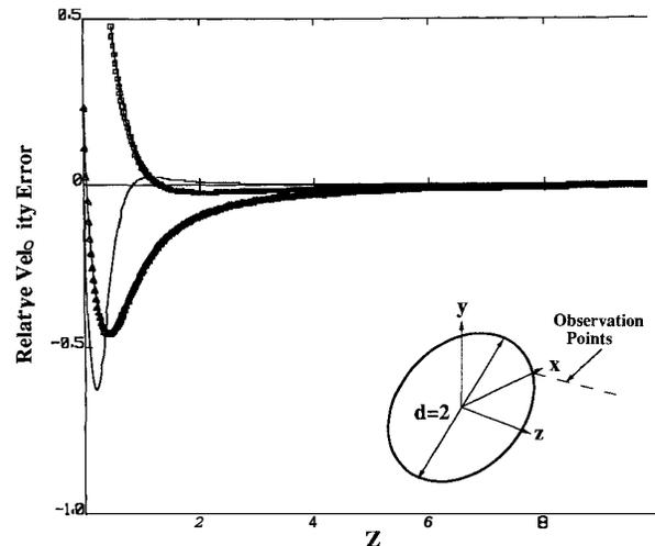
Fig. 1 Comparison of relative velocity error for multipole expansions, with one term—□; two terms—△; and three terms—solid line, computed for the vortex ring problem (insert).
