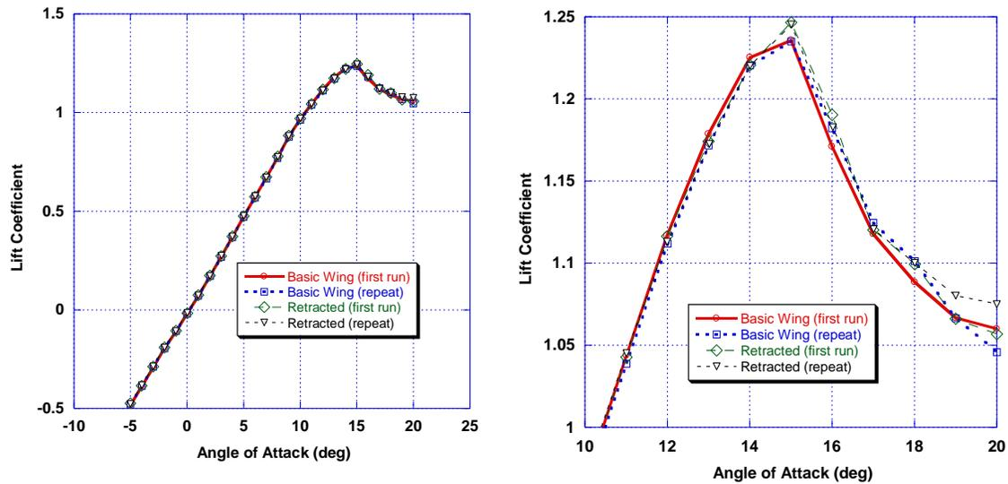
**Figure 16. (Left) lift coefficient for Basic Wing and Retracted configurations; (right) closeup of measured lift coefficients for Basic Wing and Retracted configurations in the vicinity of stall.**
