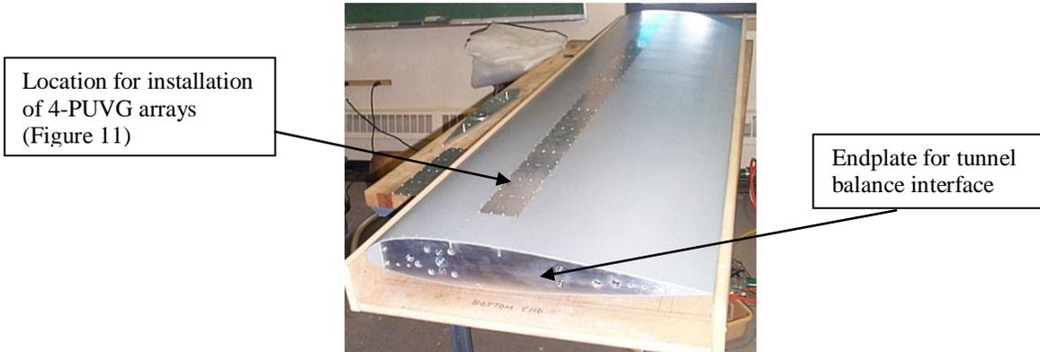
Figure 12. Fabricated wing model, in the Basic Wing configuration, prior to installation of PUVGs.
