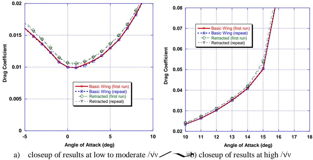
**Figure 18. Drag coefficient measured for the Basic Wing and Retracted configurations: close-ups.**
