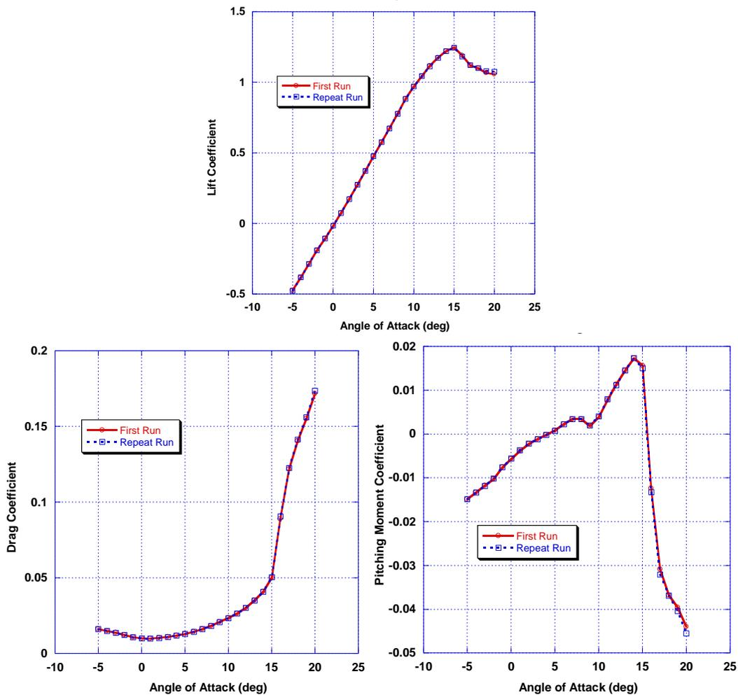
**Figure 15. Lift coefficient (above), drag coefficient (above right), and pitching moment coefficient (right) vs. angle of attack: 80 fps for the “clean” Basic Wing configuration.**
