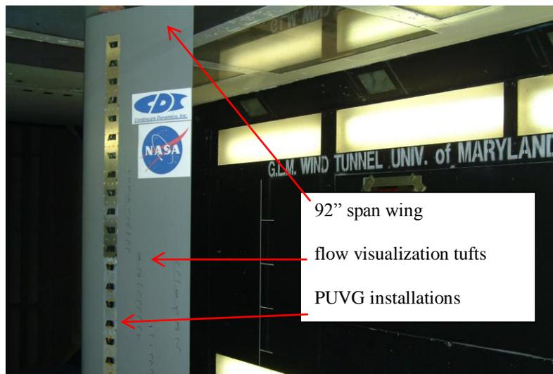
Figure 13. Overall view of vertically mounted wing model, with PUVGs installed.
