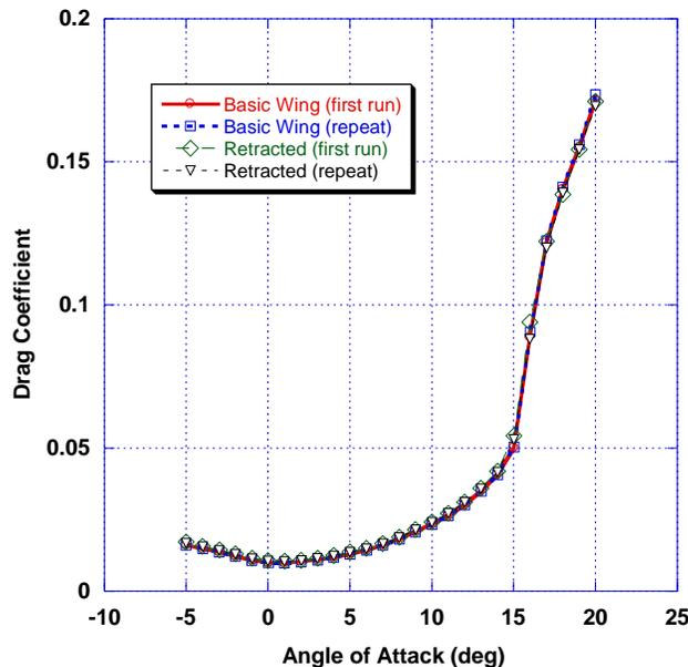
**Figure 17. Drag coefficient measured for Basic Wing and Retracted configurations.**
