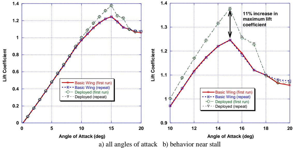
Figure 20. Effect of PUVG deployment on maximum lift coefficient.
