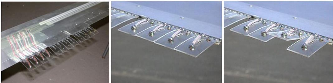
**Figure 6. A series of snap-through actuators used as trim tabs in the autogiro ground test.**
