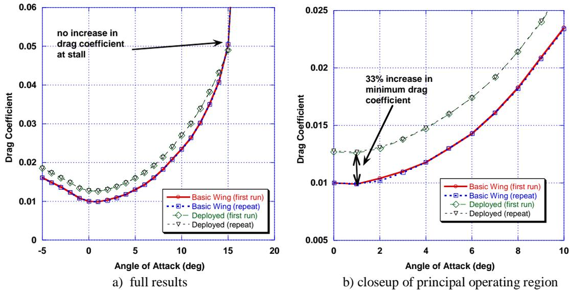
Figure 21. Drag coefficient vs. angle of attack for Basic Wing and Deployed configurations.
