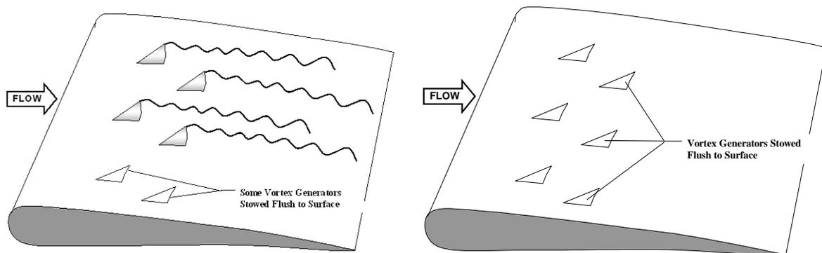
**Figure 1. Array of Pop-Up Vortex Generators (PUVG) deployed (left) and stowed (right). Note that VGs can be individually deployed and stowed.**
