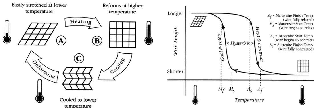
Figure 3: Schematic of SMA phase change (left) and material properties (right).
