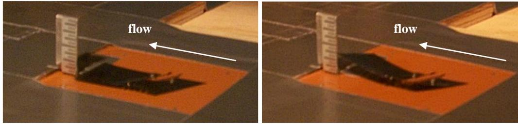
**Figure 10. Low speed wind tunnel test of deployment of an individual PUVG (120 fps flow speed; 0.25” deployed height on a 1x2” PUVG).**
