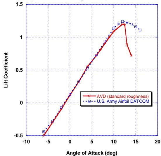
Figure 14. Lift for the NACA 23015 section (data from References 36 and 37).
