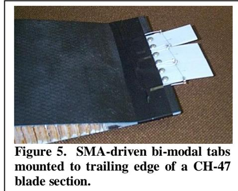
**Figure 5. SMA-driven bi-modal tabs mounted to trailing edge of a CH-47 blade section.**
