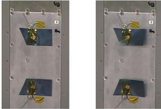
**Figure 19. Closeup of retracted (left) and deployed (right) PUVG positions for one pair of the eight powered PUVGs on the test wing.**
