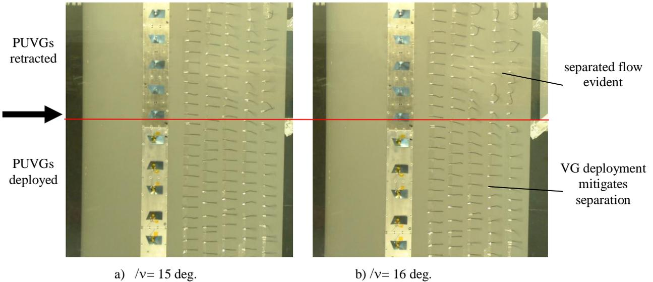
**Figure 21. Separated flow behavior and angles of attack near stall with a Partially Deployed configuration; split picture shows the effect of PUVG deployment (retracted above, deployed below).**
