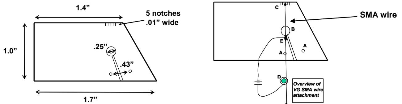
Figure 8. (left) Dimensions of initial benchtop PUVG demonstrator; (right) plan view of SMA actuated PUVG installation. (note: symmetrical wire installation providing retraction not shown)
