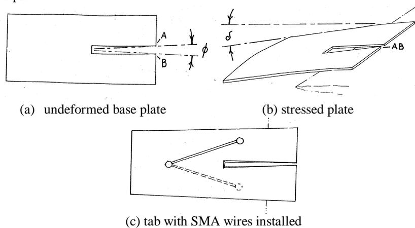
**Figure 4. Schematic of “snap-through” trailing edge tab<sup>[28]</sup>.**
