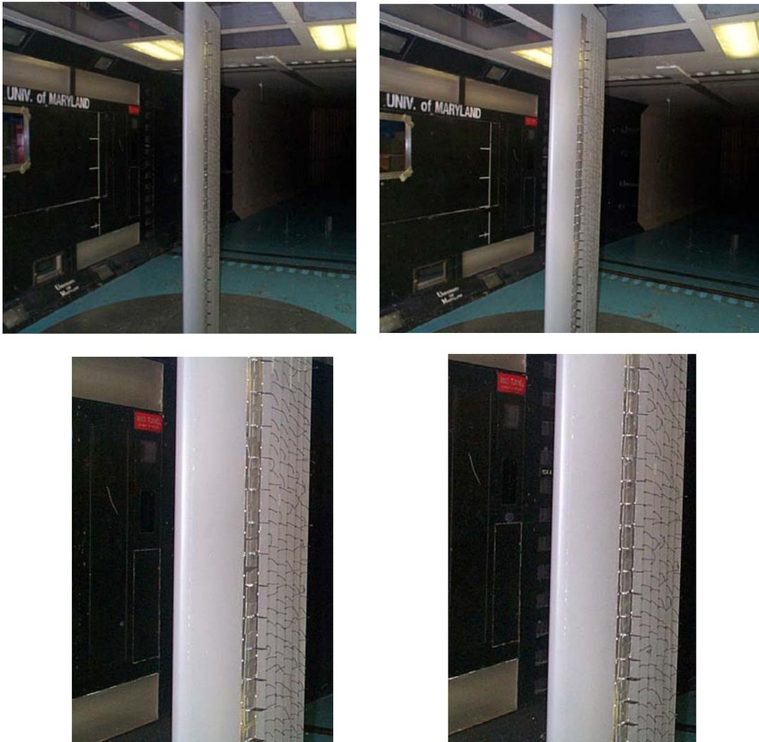
**Figure 9. Wing mounted vertically in wind tunnel with small FDOVGs installed on the suction surface; array of flow visualization tufts also shown. Left: lateral spacing = 2.3 device heights. Right: lateral spacing = 1.5 device heights.**
