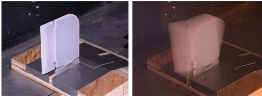
**Figure 6. FDOVG wind tunnel demonstration – left: model without flow; right: oscillating VG model operating at  $U=120$  ft/sec.**
