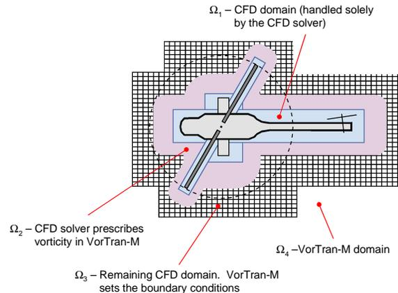
Figure 3: Detailed schematic of CFD/VorTran-M overlap regions
