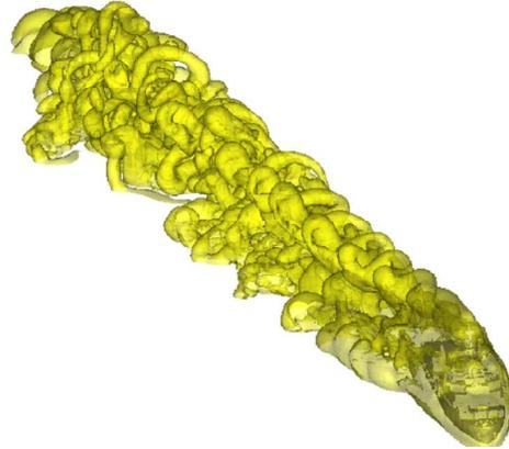
Figure 5: CGE/VorTran-M prediction of a LPD-4 class ship airwake
