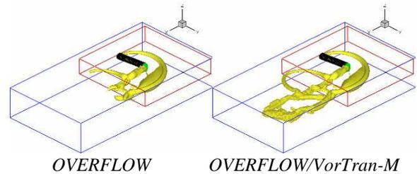
Figure 8: Predictions of wake vorticity, plotted at the same level of vorticity magnitude, for a 1-bladed rotor in forward flight after 2550 time steps
