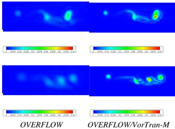
Figure 10: Predicted vorticity magnitude for a 1-bladed rotor in forward flight on a plane perpendicular to the direction of flight, 33 (upper) chord lengths and 40 (lower) downstream of the hub.  $\Delta s_{\text{OVERFLOW}} \approx 0.43c$  and  $\Delta s_{\text{VorTran-M}} \approx 0.87c$
