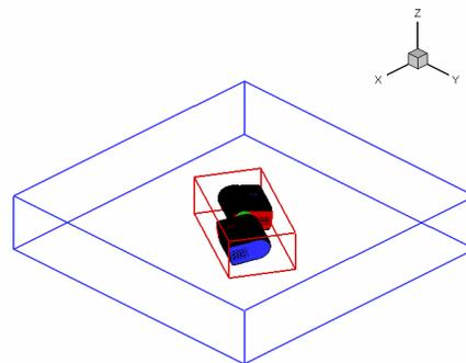
Figure 11: 2-bladed rotor and hub grid arrangement. Blade grids (black), tip-caps (blue), root-cap (red), hub grid (green), bounds of initial VorTran-M grid (blue line) and grid on which VorTran-M sets boundary conditions (red line)
