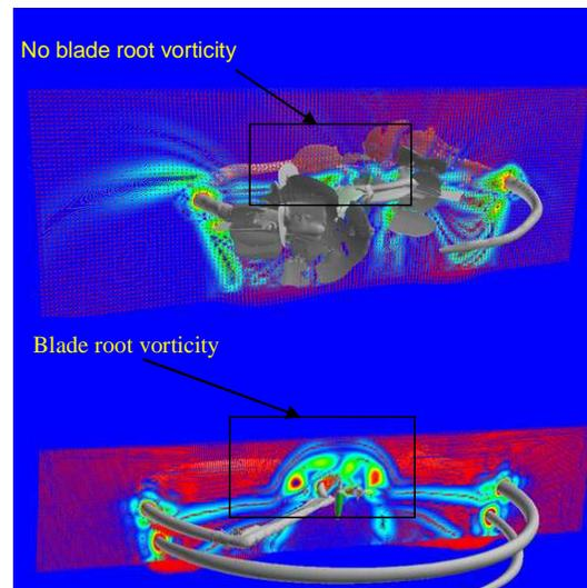
Figure 13: Close-up of OVERFLOW (upper) and OVERFLOW/VorTran-M (lower) predictions of the near-body wake and velocity vectors on a slice through the rotor
