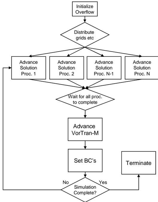
Figure 6: Overall OVERFLOW/VorTran-M coupling procedure
