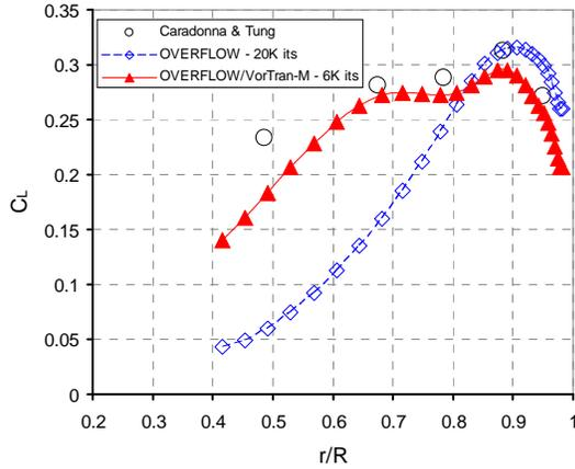
Figure 14: Comparison of measured and predicted spanwise loading ( $C_{T \text{ Experiment}} = 0.0046$ ,  $C_{T \text{ OVERFLOW}} = 0.00432$ ,  $C_{T \text{ OVERFLOW/VorTran-M}} = 0.00458$ )
