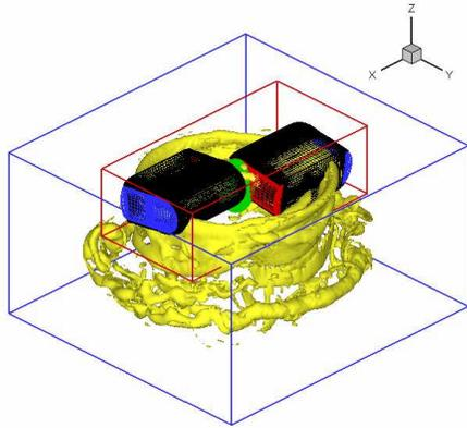
Figure 12: Iso-surface of vorticity magnitude illustrating the rotor wake predicted by OVERFLOW/VorTran-M after 5400 time steps
