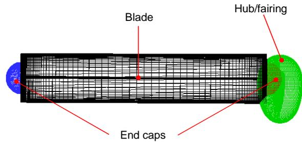
Figure 7: 1 bladed rotor and hub grid arrangement. Blade grid (black), root-cap (red) and body-of-revolution hub grid (green)
