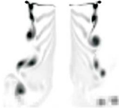
Figure 1: Snapshot of vortex pairing in the wake beneath a two-bladed hovering rotor from [48]
