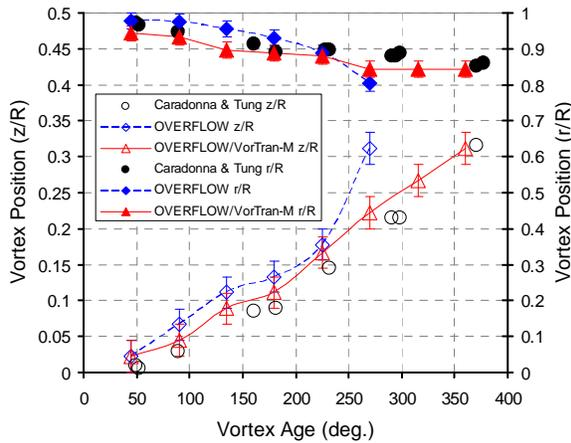
Figure 15: Comparison of measured and predicted tip vortex trajectory
