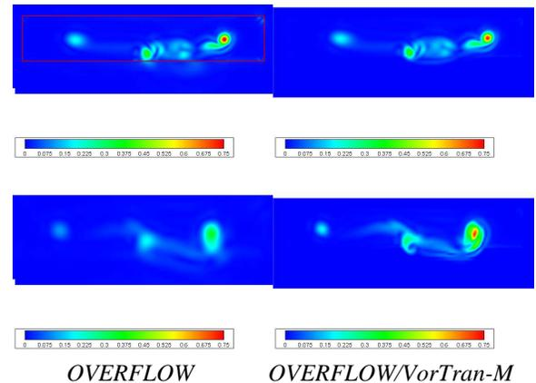
Figure 9: Predicted vorticity magnitude for a 1-bladed rotor in forward flight on a plane perpendicular to the direction of flight, 23.2 (upper) chord lengths and 31.7 (lower) downstream of the hub.  $\Delta s_{\text{OVERFLOW}}$  (red region at left)  $\approx 0.22c$ ,  $\Delta s_{\text{OVERFLOW}} \approx 0.43c$  and  $\Delta s_{\text{VorTran-M}} \approx 0.43c$
