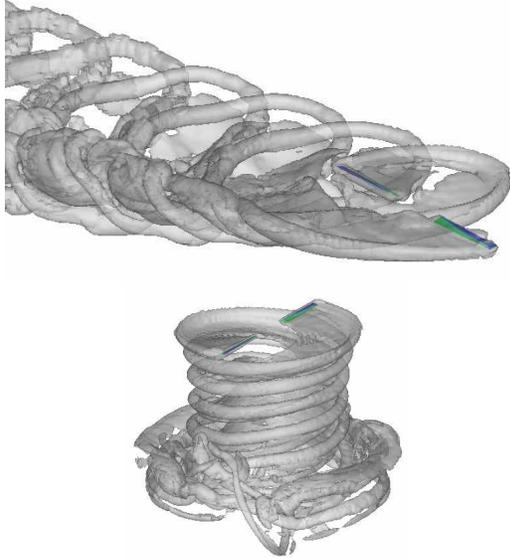
Figure 4: RSA3D/VorTran-M rotor wake predictions: two bladed untrimmed rotor in forward flight (upper) and two bladed untrimmed rotor in slow speed ascent (lower) from [44]
