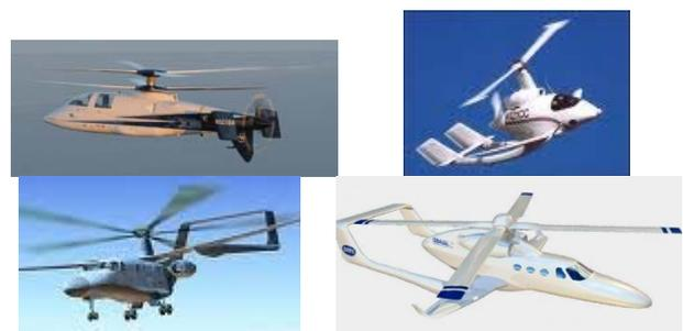
**Figure 1: High speed rotorcraft concepts (left to right): Sikorsky X2; Carter Aviation demonstrator; GBA/ DARPA Heliplane military and civil concepts.**
