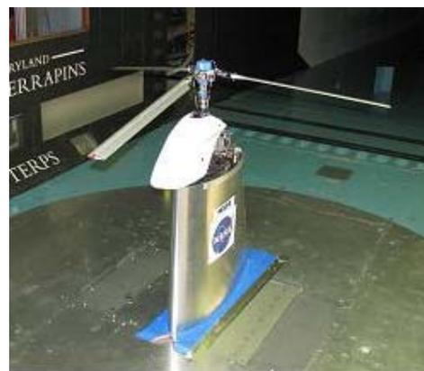
**Figure 21: New rotor test stand with torque instrumentation installed.**
