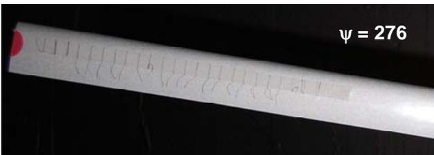
**Figure 15: Closeup view of tufted rotor blade at azimuth angle 276 deg. at advance ratio 1.7.**
