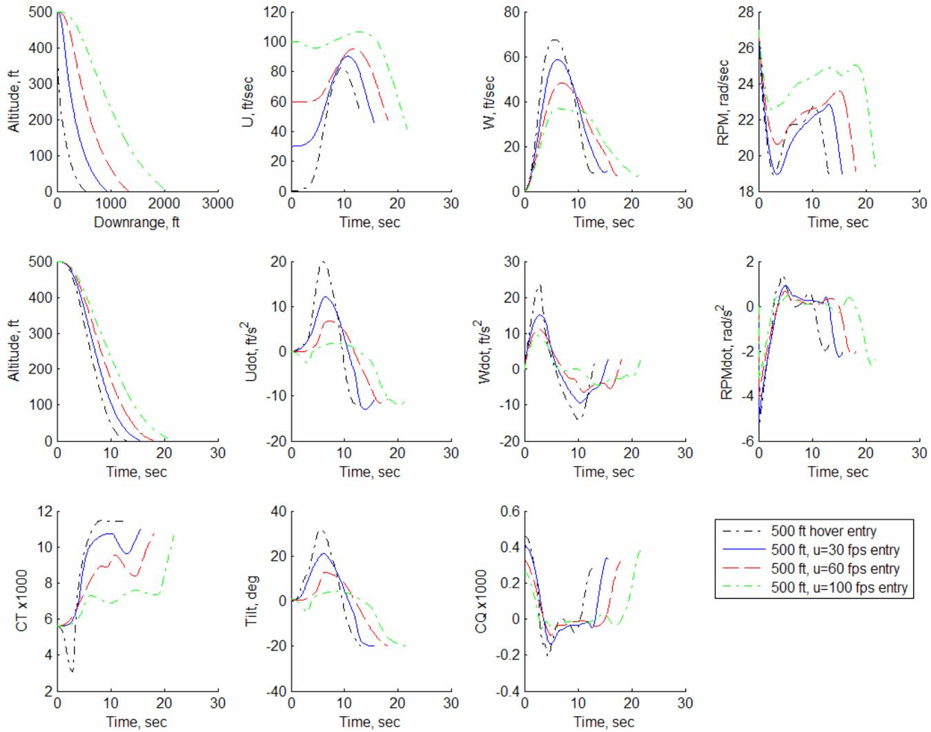
**Figure 3. H-60 Optimal Autorotation Trajectory Results (16000 lbs gross weight; 500 ft altitude entry)**
