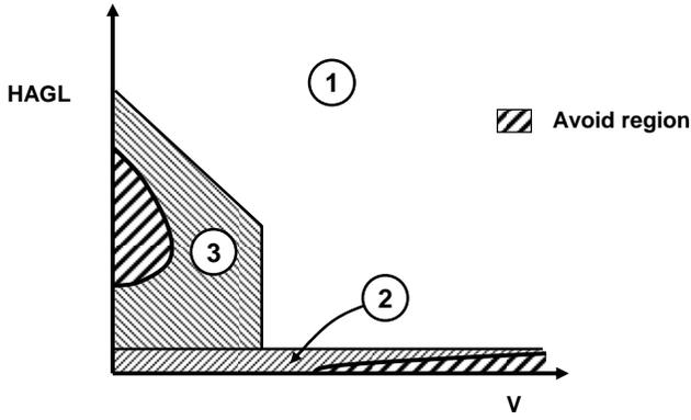
**Figure 8. Schematic Illustration of Autorotation Flight Control/Cueing Law Modes Relative to H-V Diagram**
