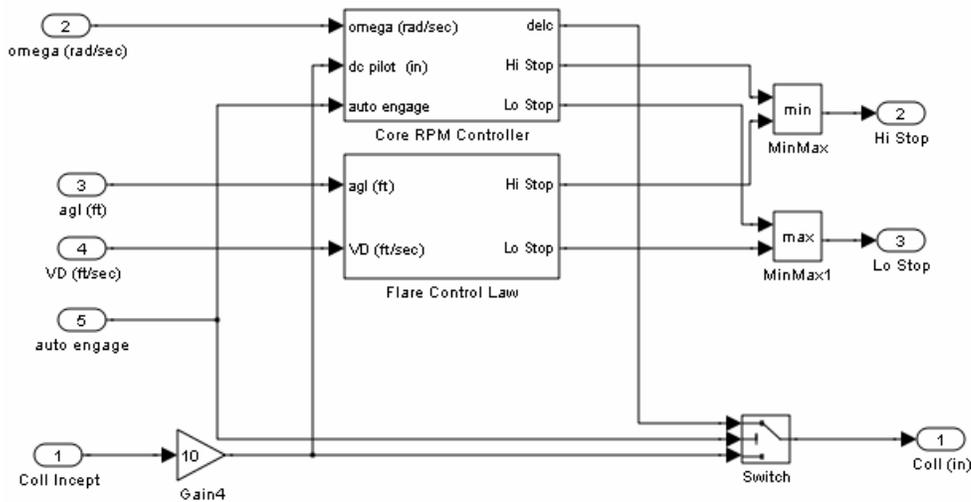
**Figure 12. Simulink Diagram for Collective Axis Control Law Used in Simulation Study**
