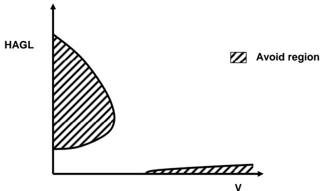
**Figure 1. Representative Autorotation H-V Diagram Illustration**
