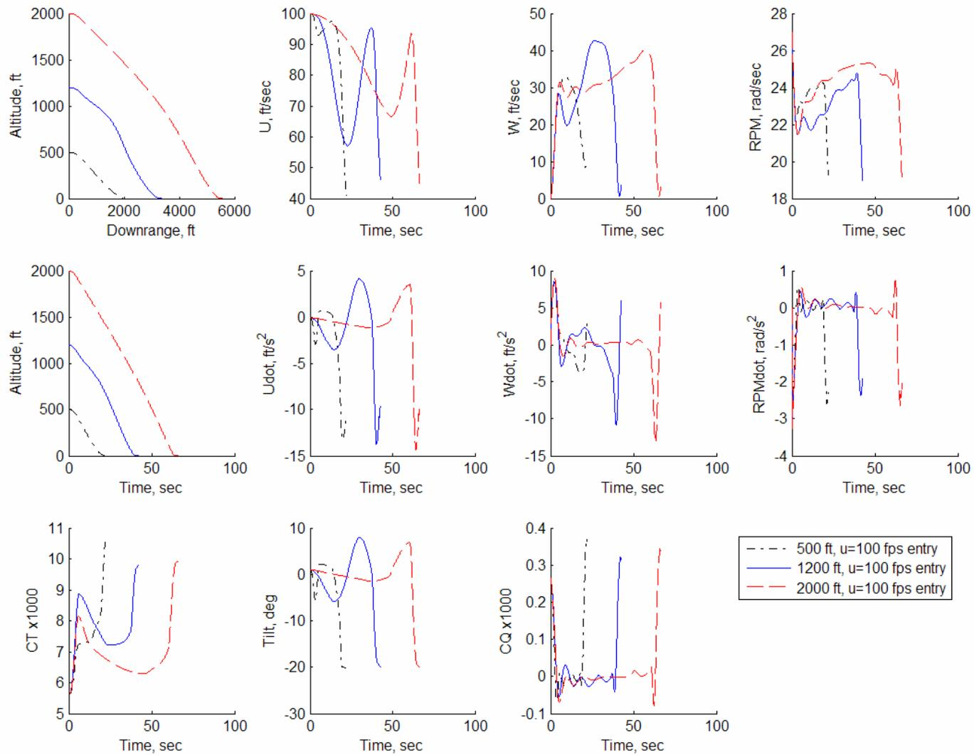
**Figure 6. H-60 Optimal Autorotation Trajectory Results with Minimum Range Performance Weight (100 ft/sec forward speed entry condition)**
