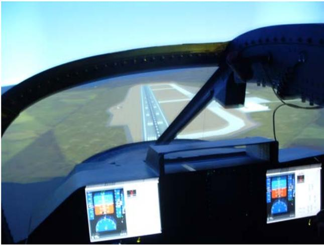
**Figure 13. Snapshot of Out-the-window View from Piloted Simulation Evaluation of Autorotation Collective Axis Tactile Cueing Law**
