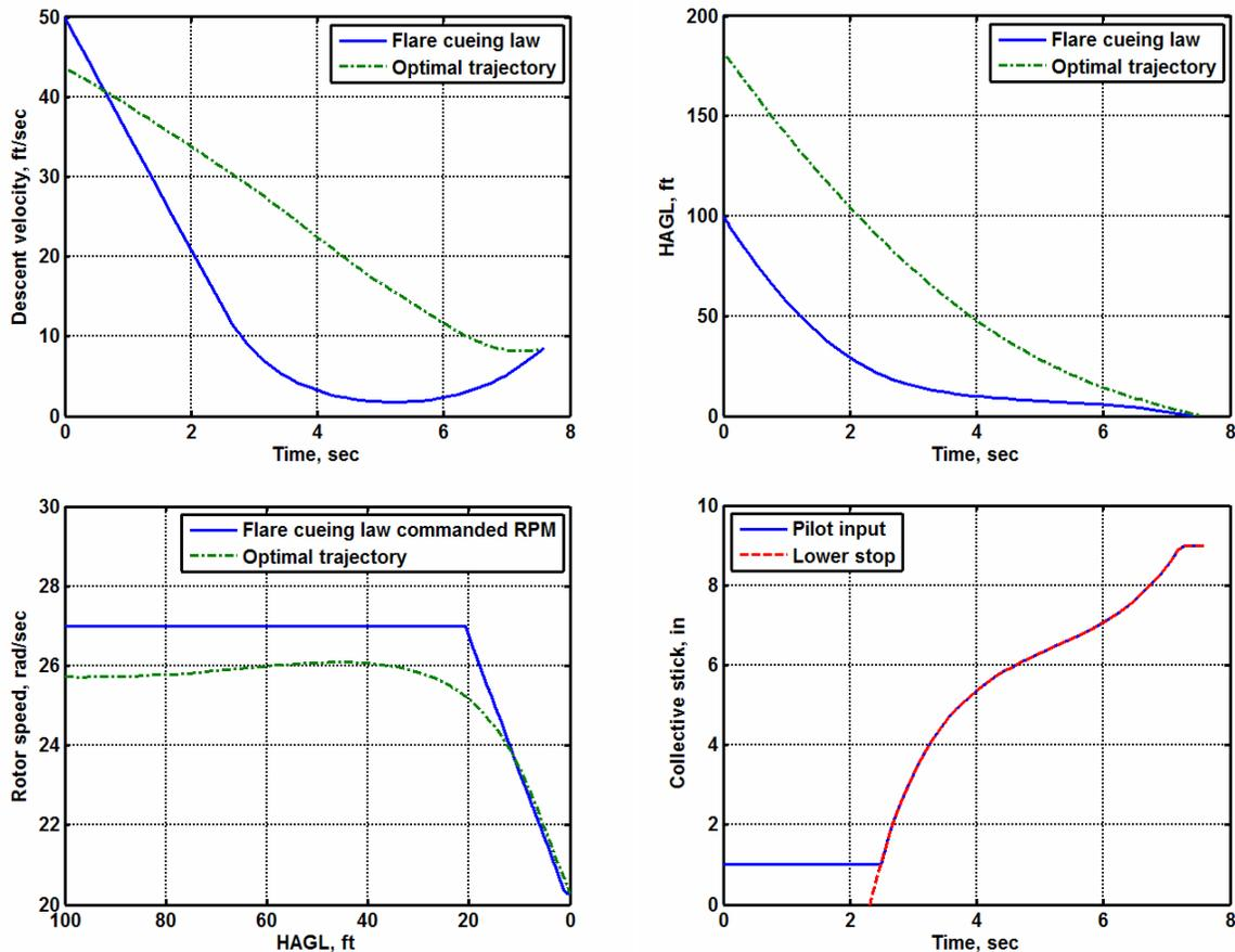
Figure 9. Comparison of Engineering Simulation Evaluation of the Baseline/Flare Autorotation Cueing Law with Optimal Trajectory Solution Results
