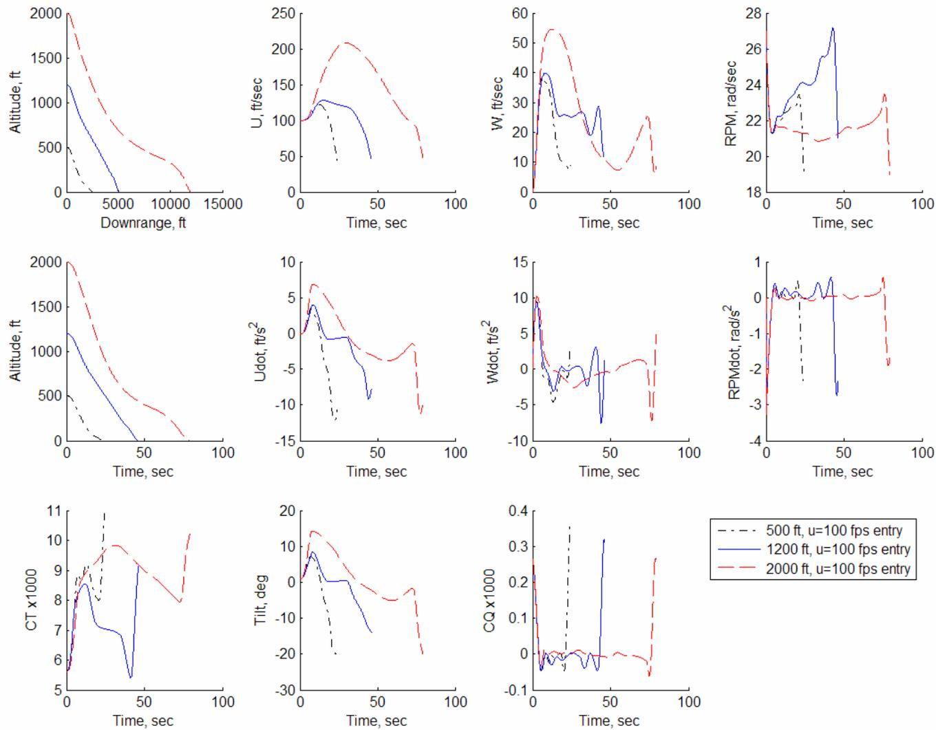
**Figure 5. H-60 Optimal Autorotation Trajectory Results with Maximum Range Performance Weight (100 ft/sec forward speed entry condition)**
