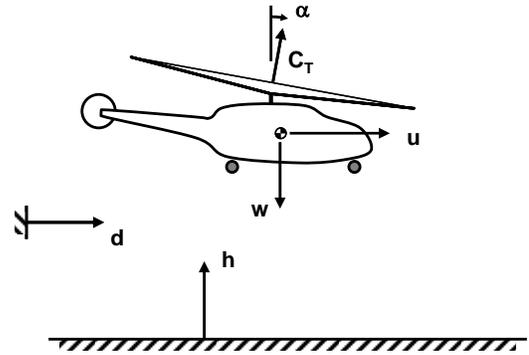
**Figure 2. Helicopter Autorotation Analysis Point Mass Model Definitions**
