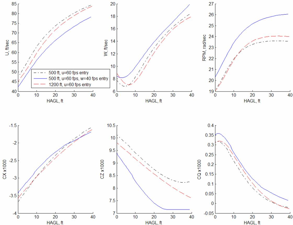
**Figure 7. H-60 Optimal Autorotation Results for Flare Segment (16,000 lbs gross weight; 60 ft/sec forward speed entry conditions)**
