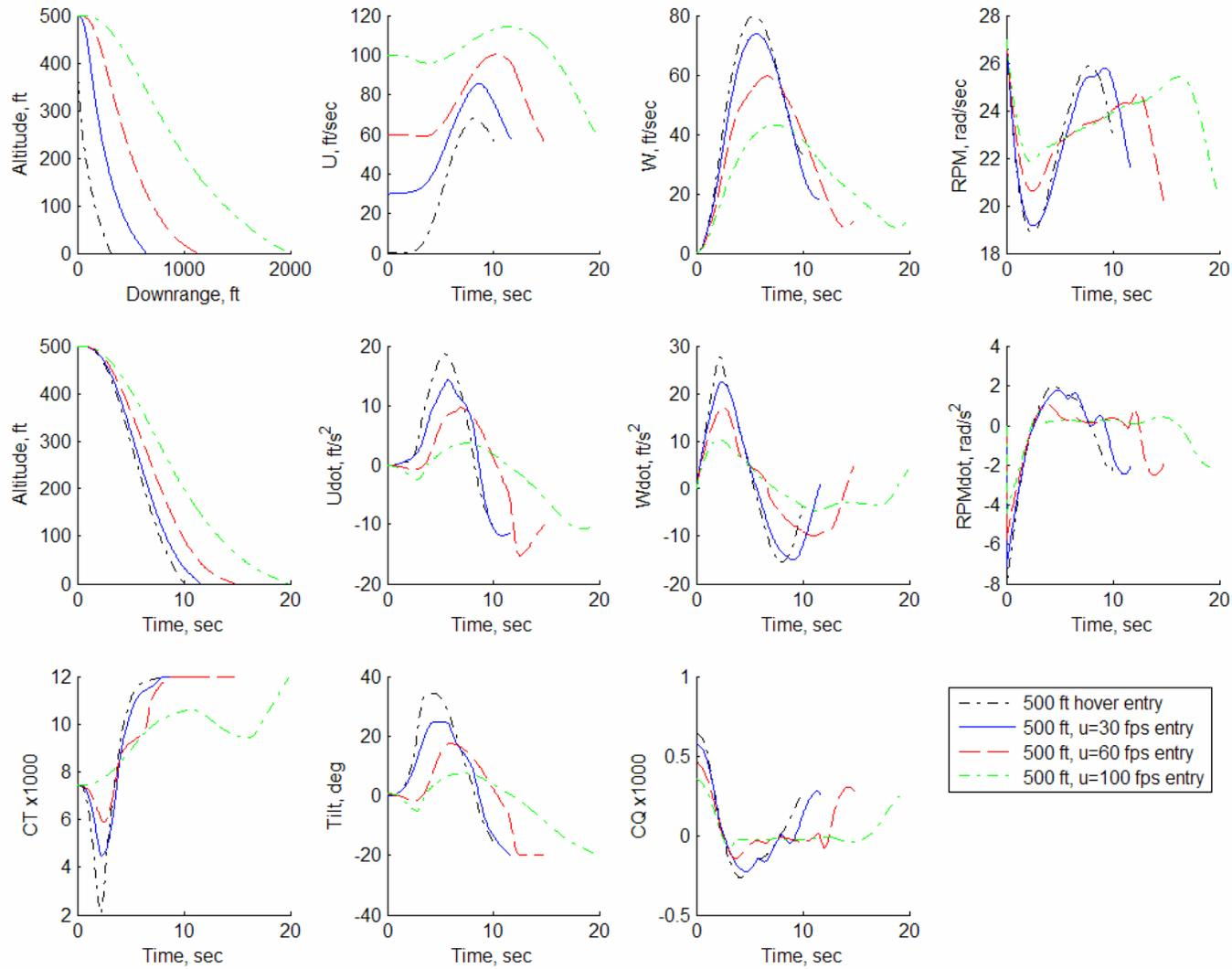
**Figure 4. H-60 Optimal Autorotation Trajectory Results (21000 lbs gross weight; 500 ft altitude entry)**
