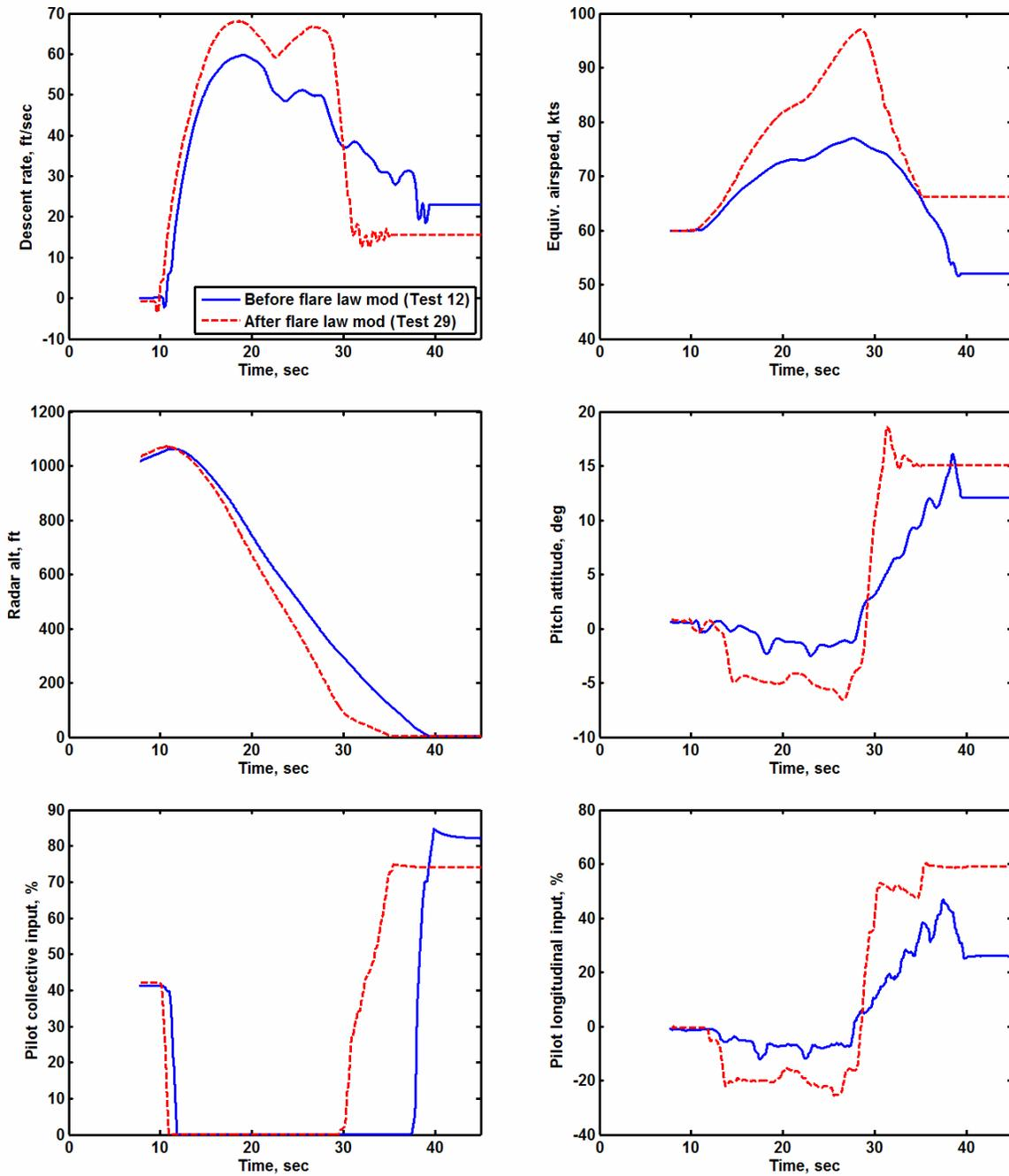
Figure 14. Representative Time Histories for Simulated Autorotation Before and After Gain Adjustment of Collective Flare Law (Pilot A)
