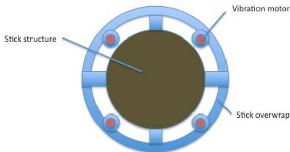
**Figure 16. Illustration of Notional Mechanical Vibration Amplification Approach for Appliqué System**
